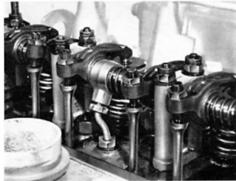
Fig. G.2. Oil Feed Pipe to Rocker Shaft.
