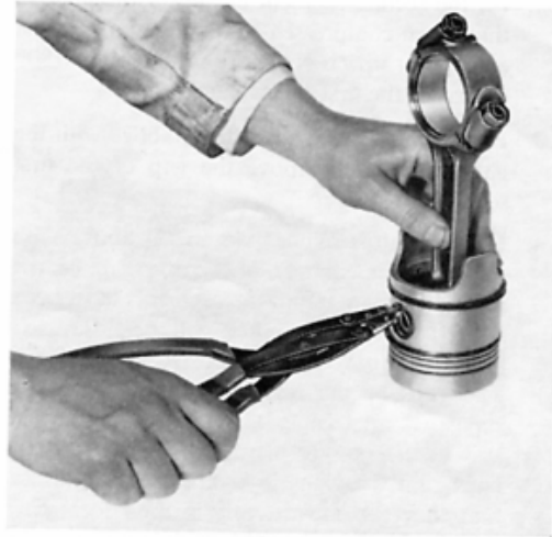
Fig. H.7. Fitting a Gudgeon Pin Retaining Circlip.
