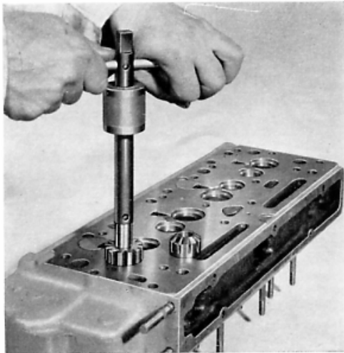
Fig. G.10. Recutting a Valve Seat.
