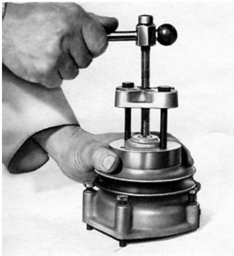
Fig. P.4. Removing the Water Pump Pulley.
