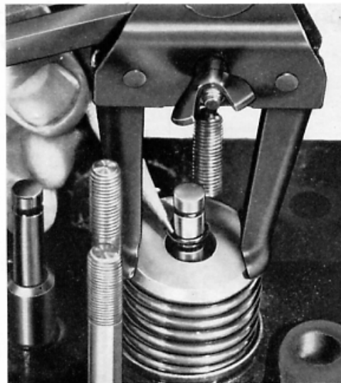
Fig. G.18. Locating a rubber 'O' Ring.
