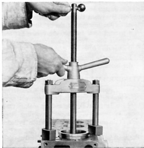
Fig. J.4. Removing Cylinder Liner.
